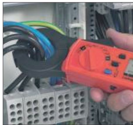
Differential current measurement with leakage current clamp
