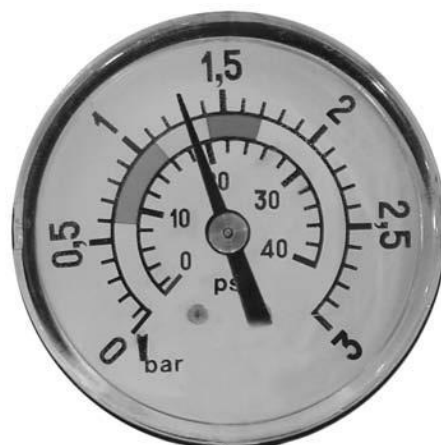
1,3 kg/cm 2 - 18,5 PSI: This pressure indicates that it is necessary to "BACKWASH".
